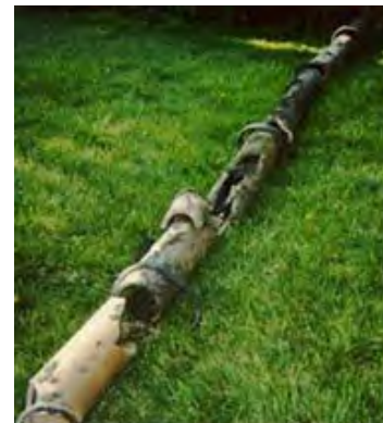
Figure 4-4: Home Lateral Infiltration
