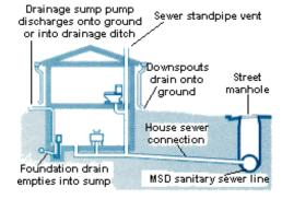
Stop the inflow and infiltration by disconnecting downspouts and sump pumps from sewer the system
