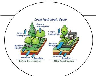
Increased impervious surface causes increased stormwater runoff
